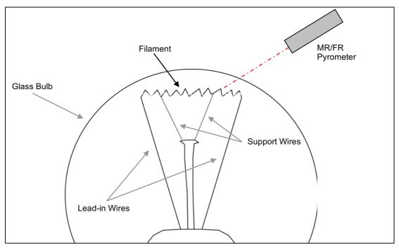
Temperature Measurement of the Filament as a Function Control of the Light Bulb
