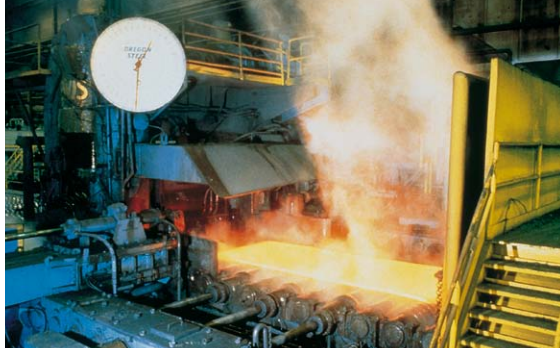
Accurately measuring temperature of slabs, billets, or blooms on a hot rolling mill ensures consistent product quality.
